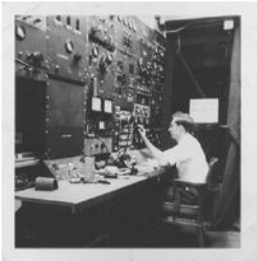
Karl Brown at the klystron controls for the Mark II accelerator at Stanford University
